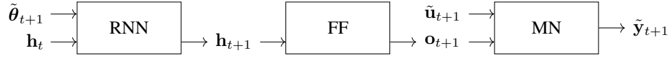
Figure 8: A schematic representation of the LRNN surrogate family for a single time step. First, the parameters \tilde{\theta}_{t+1} are passed to a recurrent neural network (denoted by RNN in the diagram) that updates its hidden state. The updated hidden state is passed to a feedforward neural network (denoted by FF in the diagram), which computes the logits \mathbf{o}_{t+1} for a multinomial distribution from which \tilde{\mathbf{y}}_{t+1} is sampled.
